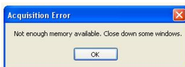
Figure 1 – “Not enough memory available” Error message appears when acquisition is likely to exceed available PC RAM
